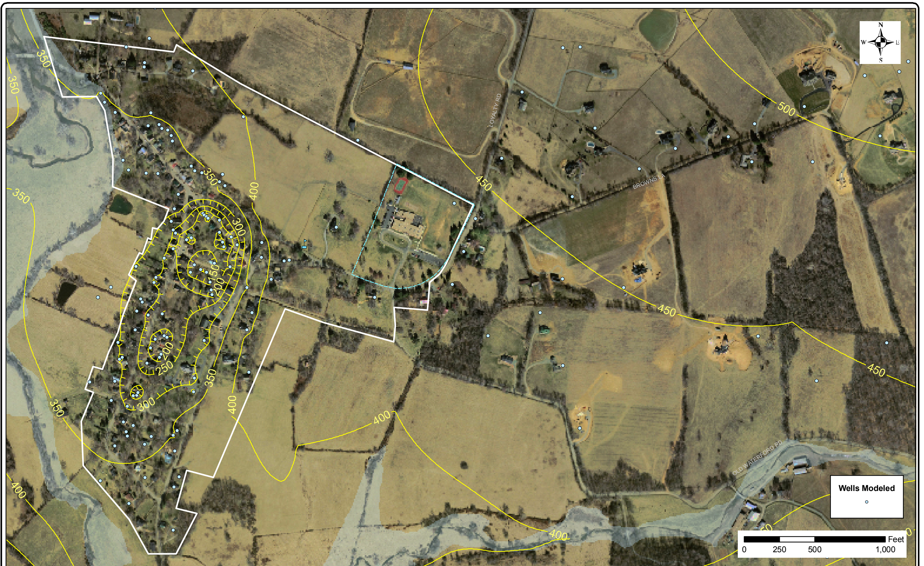
Figure 29. Simulated steady-state hydraulic head values contoured in feet above MSL (run WF-SS-1). Model results are based on a simplified representation of the existing condition. Each well was pumped at a rate of 125 GPD in the simulation, discharge from the spring near Butchers Row was set at 2880 GPD, and 644 GPD were pumped from the WES well.
