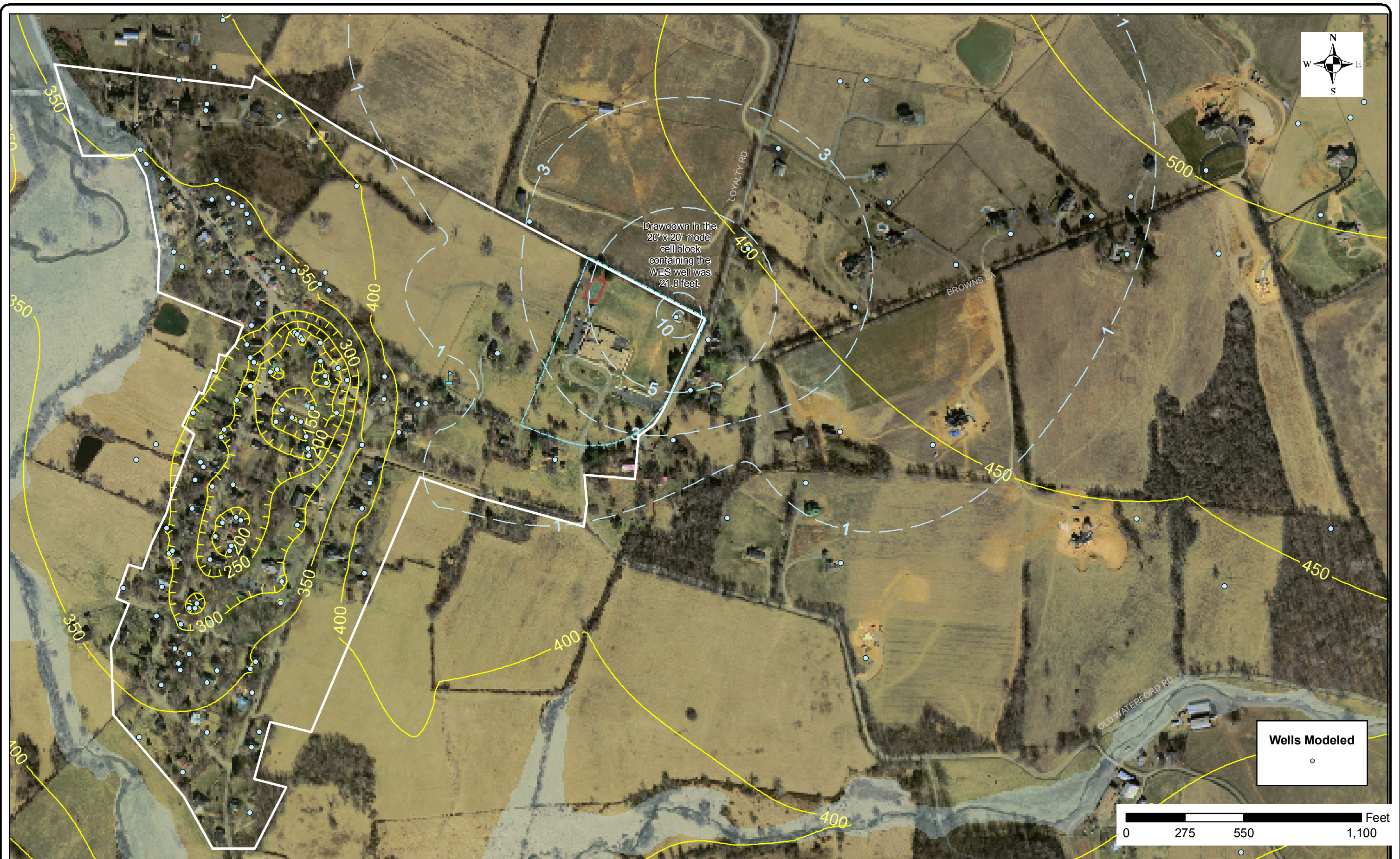
Figure 30. Simulated (run WF-SS-2) steady-state hydraulic head (yellow) and drawdown (light blue) contours in feet resulting from increasing the pumping rate at the WES supply well from 644 GPD to 2349 GPD. Model results are based on a simplified representation of hydrogeologic conditions. Other wells were pumped at a rate of 125 GPD each in the simulation, and 2880 GPD were discharged from the spring near Butchers Row.
