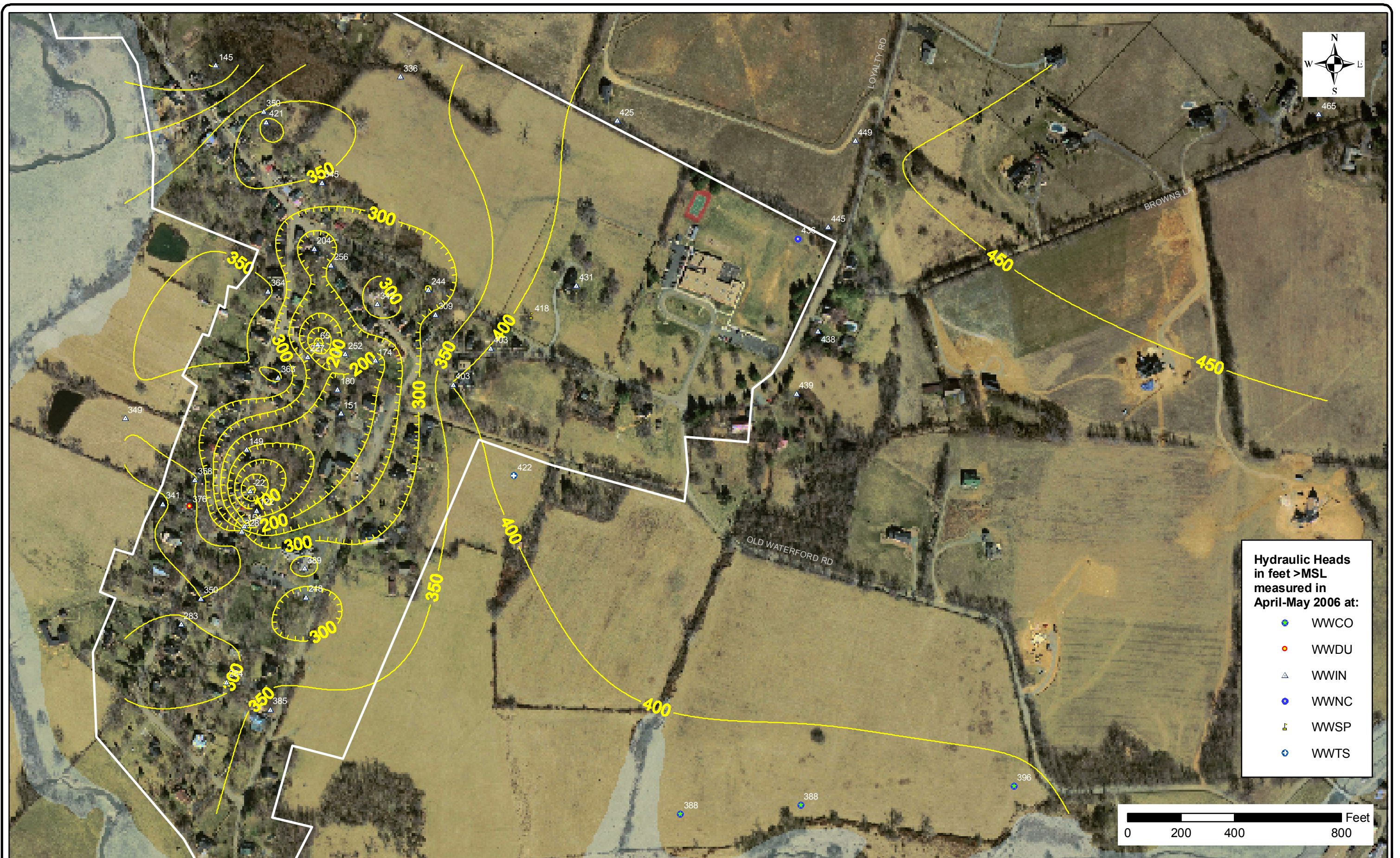
Figure 5. Hydraulic head values posted and contoured in feet above MSL based on measurements of depth-to-water in water wells during April and May of 2006. Note that nearly all of the wells are pumped to provide domestic water supplies. Contours (50-ft) were interpolated by kriging using a 5-ft cell size.
